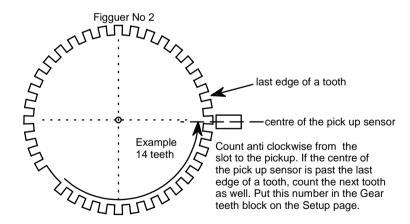
In this example the slot is past a quarter of the gear. This means that the ECU will fire on coil 4 first, then on coil 1, then on coil 2 and then on coil 3. This setting will be 14 teeth - 9 teeth = 5 teeth and then about 4 degrees for the BTDC setting. For a 60-2 gear the subtract value is 15 instead of 9.
