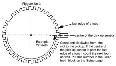
In this example the slot is past a half of the gear. This means that the ECU will fire on coil 3 first, then on coil 4, then on coil 1 and then on coil 2. This setting will be 22 teeth - 18 teeth = 4 teeth and then about 6 degrees for the BTDC setting. For a 60-2 gear the subtract value is 30 instead of 18.
