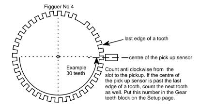
In this example the slot is past a half of the gear. This means that the ECU will fire on coil 3 first, then on coil 4, then on coil 1 and then on coil 2. This setting will be 30 teeth - 27 teeth = 3 teeth and then about 2 degrees for the BTDC setting. For a 60-2 gear the subtract value is 45 instead of 27.
